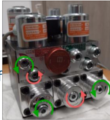
KLEEMANN Valve block that controls the lift
