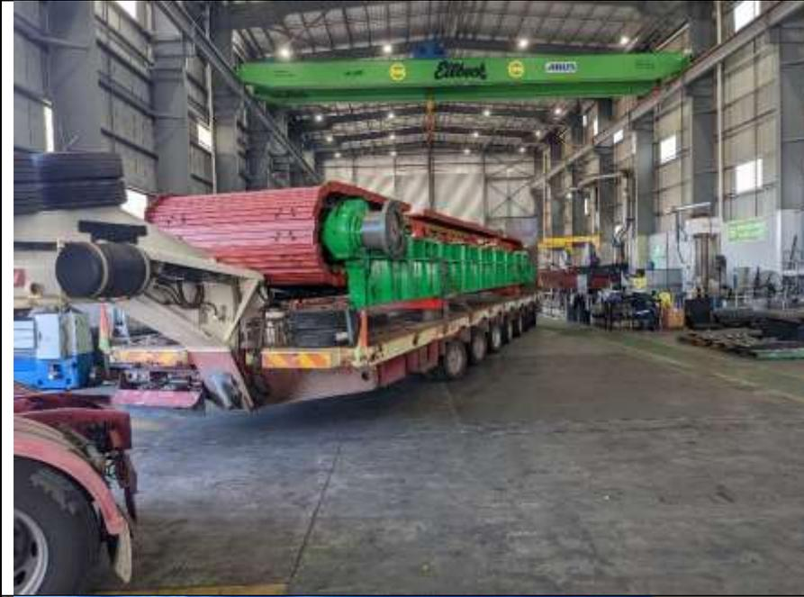
The MMD sizer being assembled ready for transportation to Laos.
